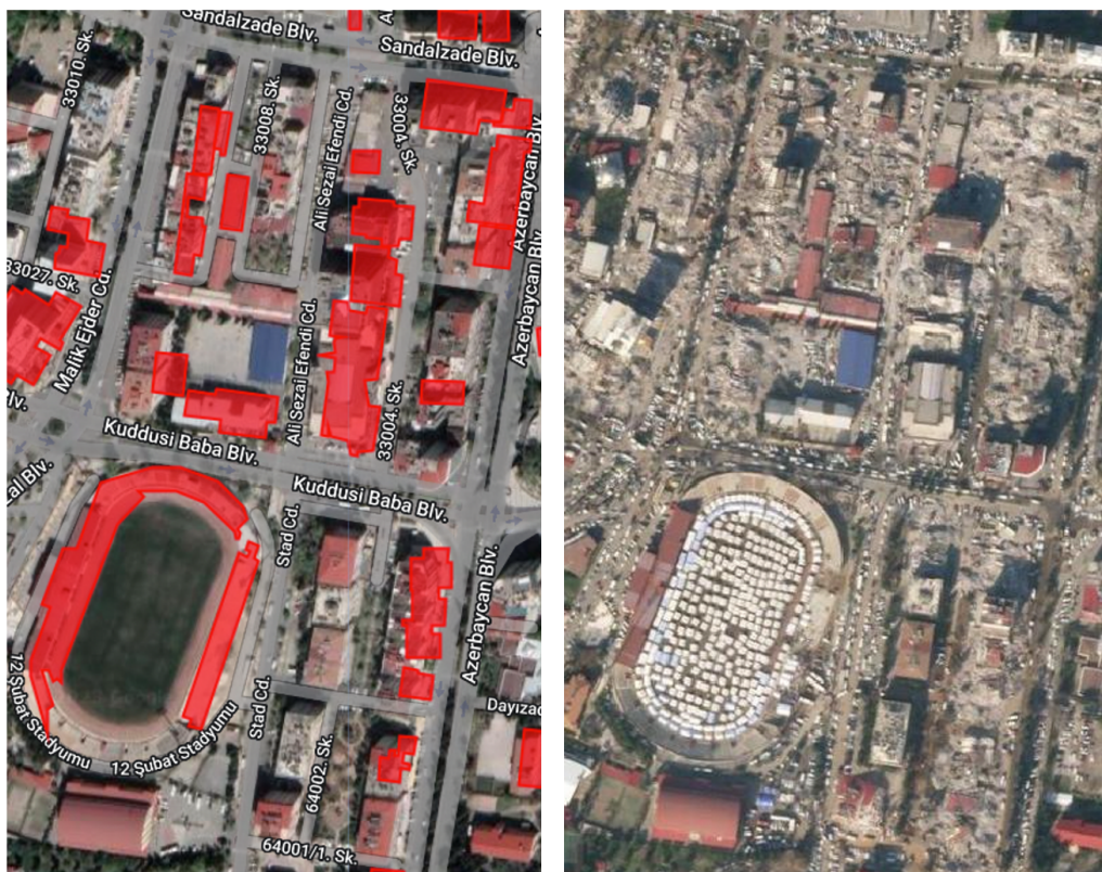
Figure 5: Predicted damaged buildings in Turkey and High-Resolution image
